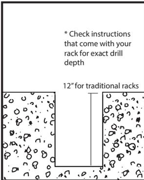
1. Use the auger to drill the hole or holes for installing the racks into the starting base material to the depth recommended for your specific racks installation - 12" is standard for traditional style bike racks
